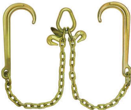
V-Chain with Classic Style 15" J Hooks 5/16" Chain. Grab Hooks at Pear Link
