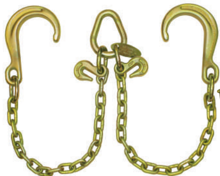
V-Chain With Classic Style 8" J Hooks 5/16" Chain. Grab Hooks at Pear Link
