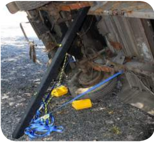
Rollover Stabilization Kit Includes 2-Ratchet Straps and 1- 4" x 4" x 6" Shoring Crib with Handle
