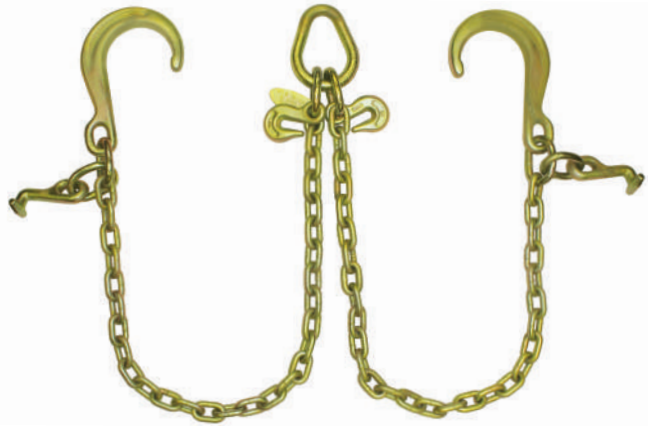
G70 V Chain with Classic Style 8" J & T Hooks 5/16" Chain. Grab Hooks at Pear Link
